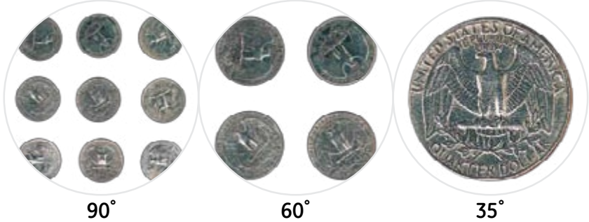
The 90° field-of-view, shown at the far left, produces the lowest magnification. The 60° and the 35° field-of-view provide increasingly greater magnification.
